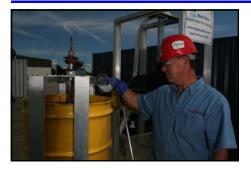
Add polymer to mix tank at dose rate determined by Rapid Dewatering Test (RDT)
